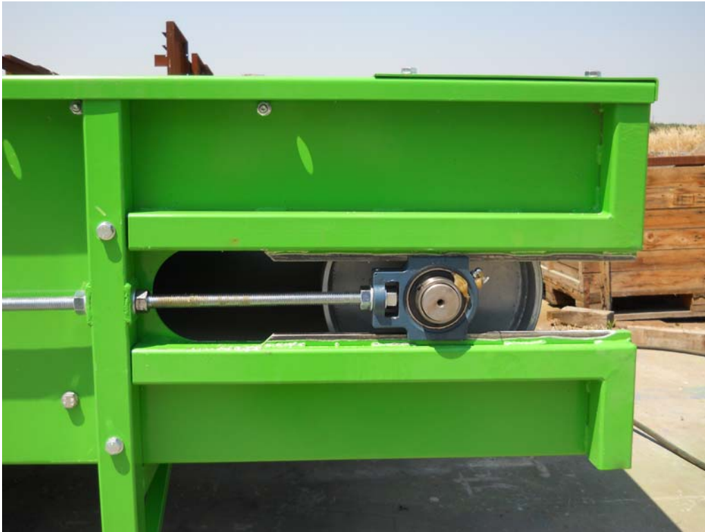
Figure 11 - Bearing support of idle roller
